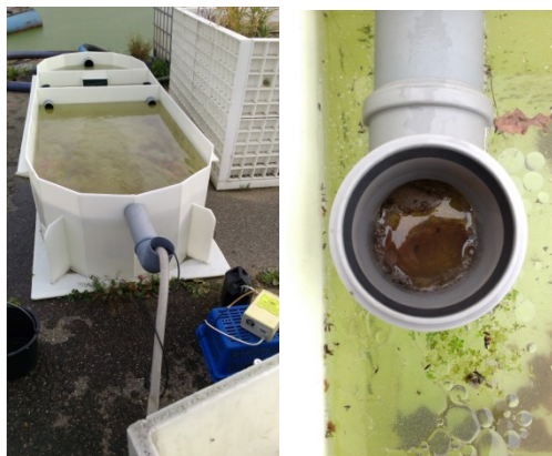
Figure 2a,b. Semi-operated model of DUN storm water tank (left). Accumulation of oil substances at the water surface during validation testing (right).
