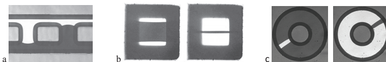
Fig. 1. Microphotographs of sensitive elements saturated in opposite directions: a – bridges 30 \times 60 \mu\text{m} , b – squares 60 \times 60 \mu\text{m} , c – rings 90/30 \mu\text{m} .
