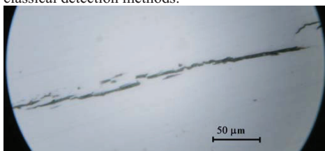
Figure 1. Macrograph (200X) of a region with crack. The opening of the crack is in the micrometer range.
