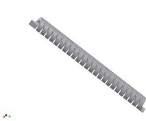
Figure 1 : « helicore » of the orthogonal induction sensor.
